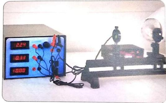
3. Vary the Voltage across LDR ranging from 0 to 5V. Note the Voltage and Current in voltmeter and ammeter at different intervals.
