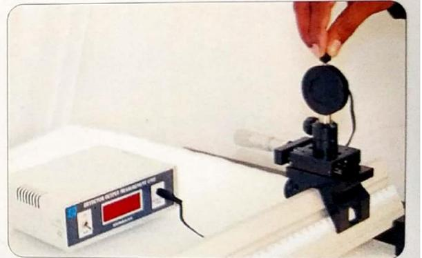
6. Switch on the laser and Output measurement unit. Align the crystal and laser so that laser beam is parallel to the face of the crystal. Adjust the kinematic setup provided on the laser mount to get the beam in the field of standing wave generated.
