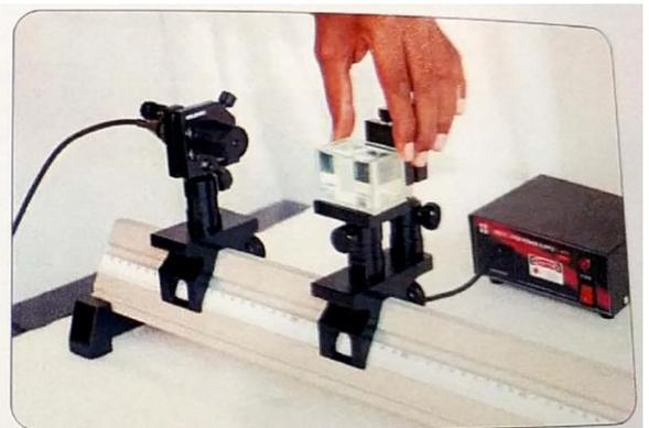
4. Fix the crystal on the mount and keep it immersed fully in the liquid. Connect it to the RF oscillator.
