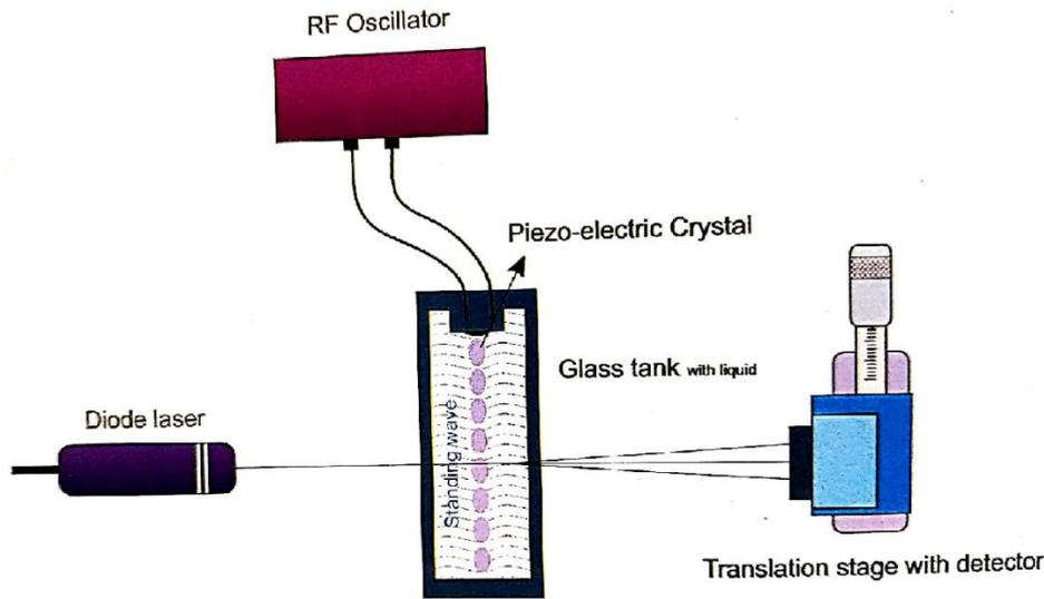
The ultrasonic waves generated by the transducer travels down the medium (liquid), gets reflected at the bottom (flat glass plate) of the cell. The incident and reflected waves interfere and stationary/ standing waves pattern is formed. The velocity of ultrasonic waves in a liquid is calculated using the formula:
