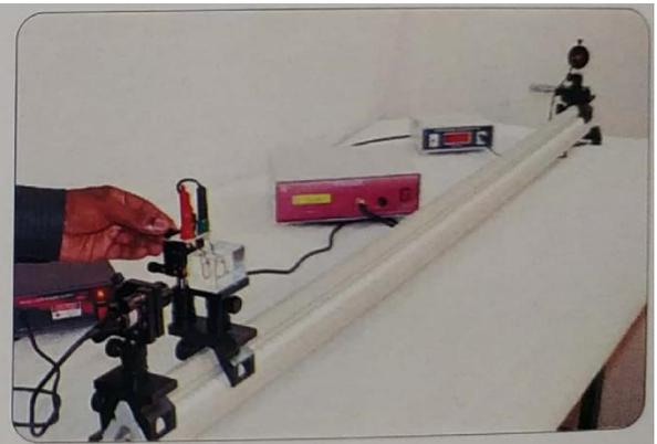
7. Keep the laser spot falling on detector stage and adjust the frequency of the oscillator until you get a very good fringe pattern on both sides of the central
