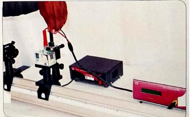
5. Fix cell mount with linear translation stage on the rail. Insert the pinhole detector into the cell mount and connect the output probe to measurement unit.
