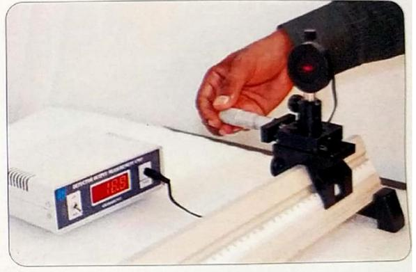
8. Scan the pattern at close intervals. Each time note the micrometer reading and corresponding output of the detector.
