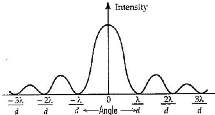
Figure 2 Diffraction pattern obtained through single slit
