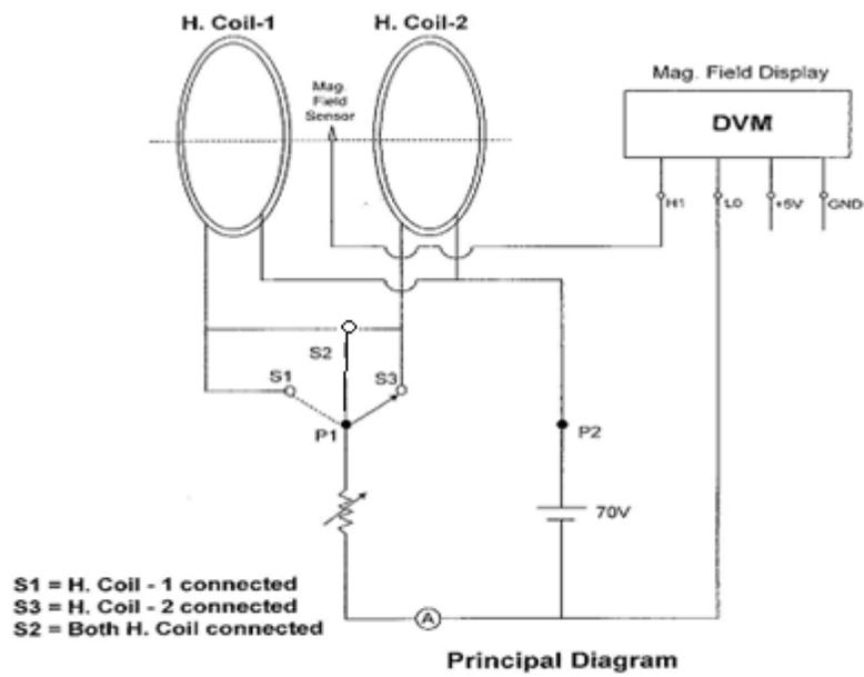
**MAGNETIC FIELD MEASUREMENT APPARATUS**
