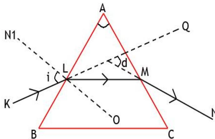
As the angle of incidence is increased, angle of deviation ' $d$ ' decreases and reaches minimum value. If the angle of incidence is further increased, the angle of deviation is increased.
