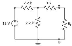
If you remove the load resistance  $R_L$  and measure the open circuit voltage across terminals A-B (VOC) with the help of a digital multimeter, ideally what should be the value displayed on the multimeter (Take resistances in Ohm and k in the diagram means kilo)?
