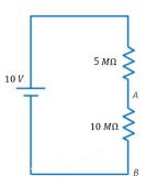
The reading on a multimeter on measuring the voltage across node A and B is 5 V. Theoretically, the voltage across A-B is  $\frac{20}{3}$  V. What is the problem with the measurement, considering the multimeter is not-faulty?
