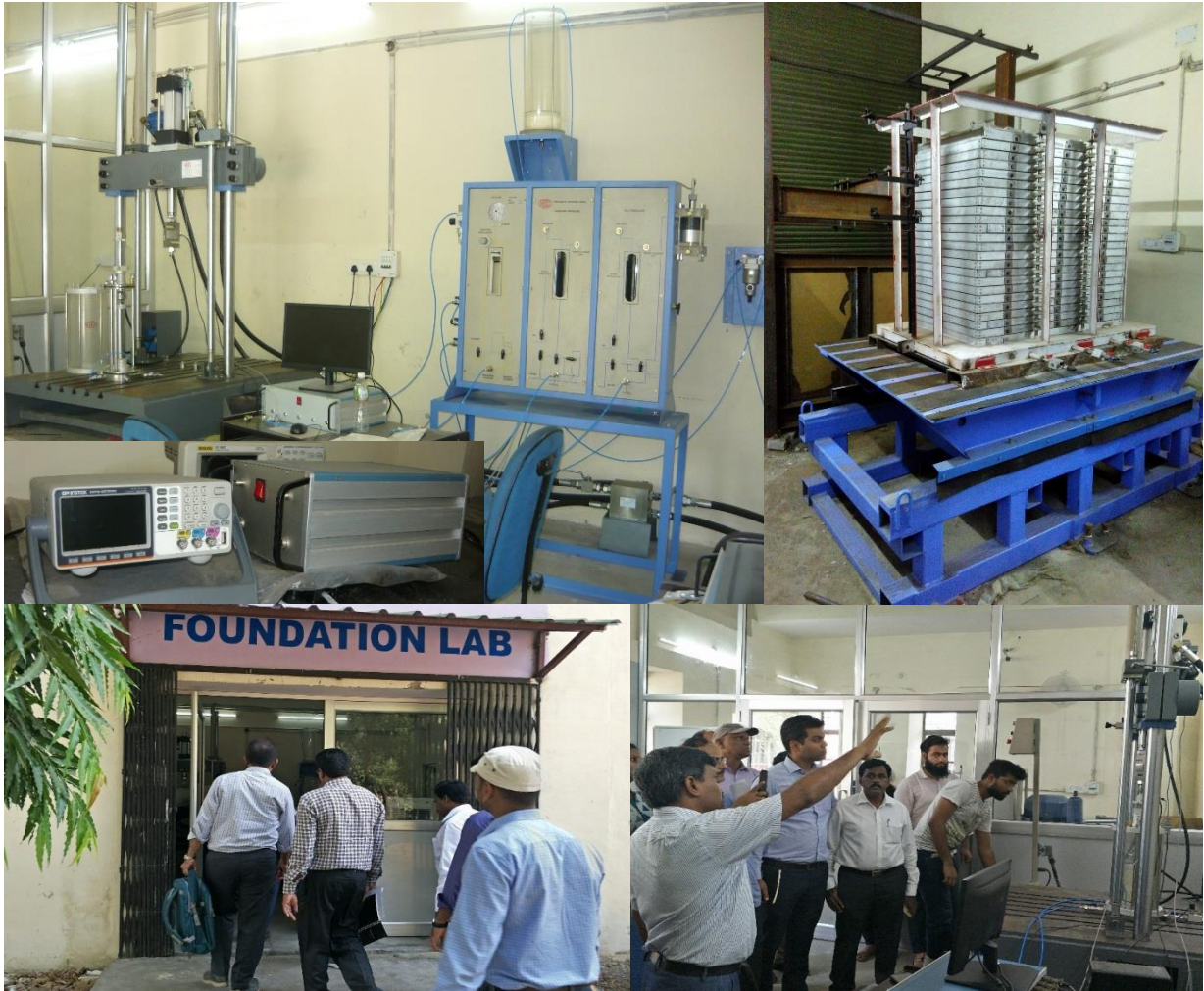
Picture.1 - Large Size Cyclic Triaxial Machine & Servo Controlled Uni-axial Hydraulic Shake Table at Foundation Engineering Laboratory, Dept. of Earthquake Engg.
