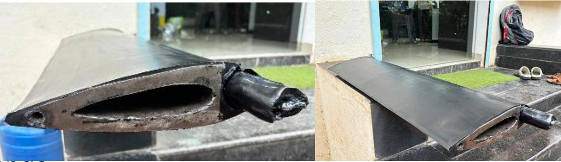
A. Thermoplastic and Steel Combination blade
