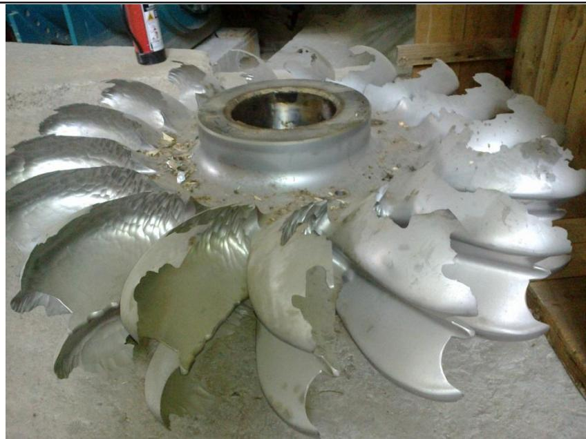
Eroded Pelton wheel of
