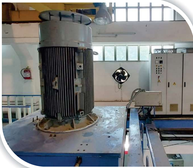
Dynamometer on movable trolley driven by VFD (SINAMICS S120-Siemens)
