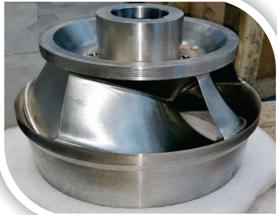
Model Pump Turbine Runner
