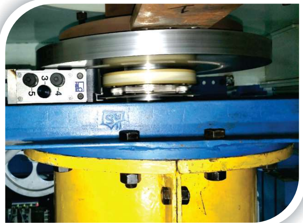
Measurement of Turbine Speed by rotary Speed transducer
