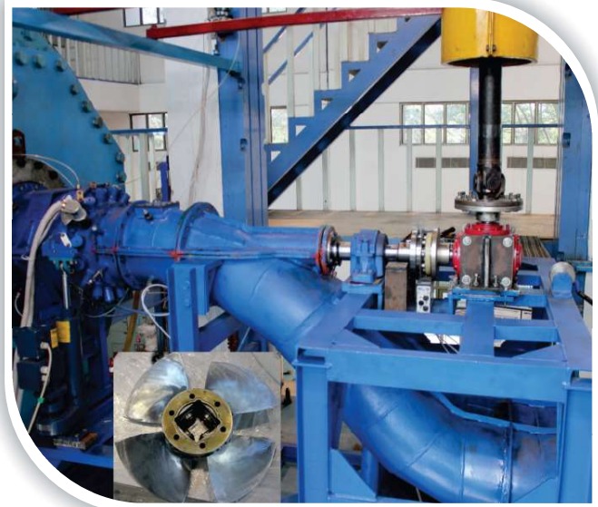
Horizontal Kaplan model with Bevel Gearbox
