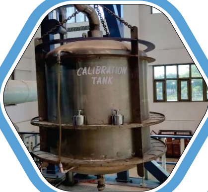
Calibration tank with load cell
