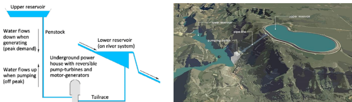
(b) Off-stream open loop pumped storage scheme
