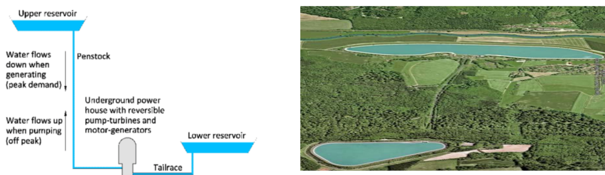
(c) Off-stream closed loop pumped storage scheme
