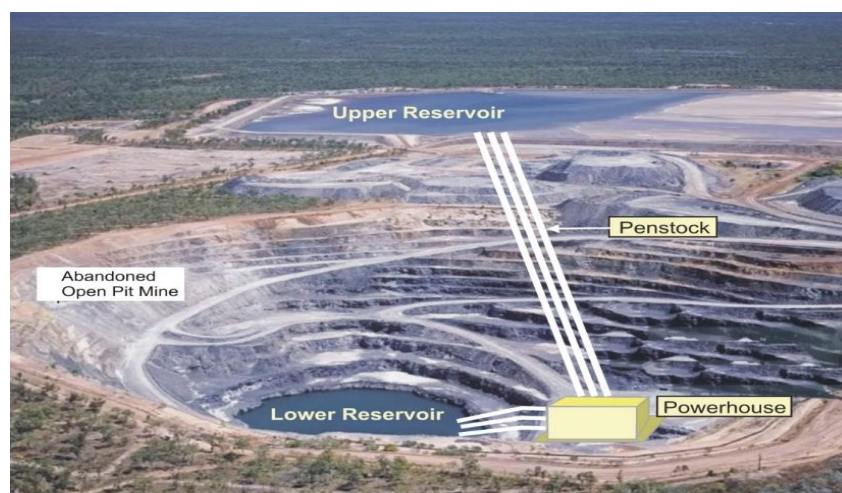
Figure 2.7: A conceptual layout of a PSP in abandoned Open-pit mine
