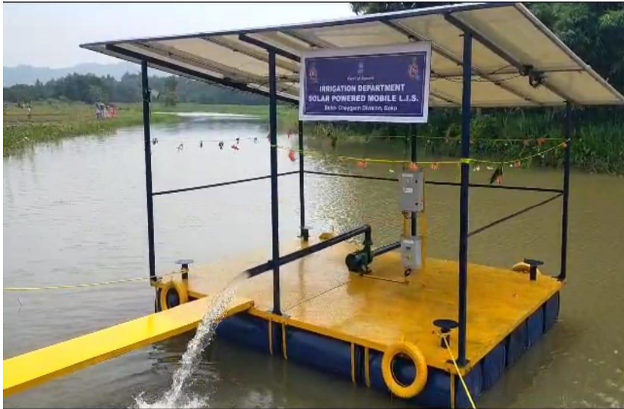
Fig. 5: Solar-powered mobile lift irrigation scheme in Boko, Assam. (Source: National Water Mission, Ministry of Jal Shakti, Department of Water Resources, RD & GR, Government of India).
